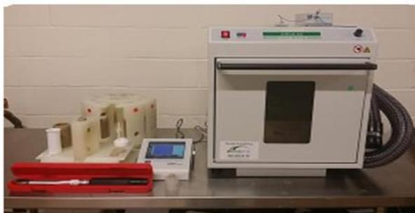
**Figure 1:** Microwave assisted milestone start D digester.
