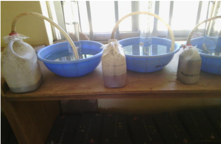
Figure 4: Experimental setups for the effect of digester size on biogas production
