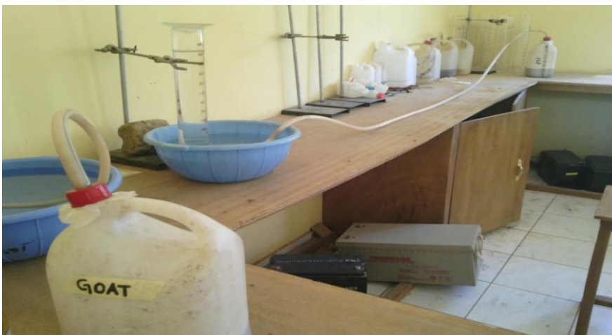
Figure 2: Experimental setups for the effect of distance traveled by the gas on the efficiency of biogas production
