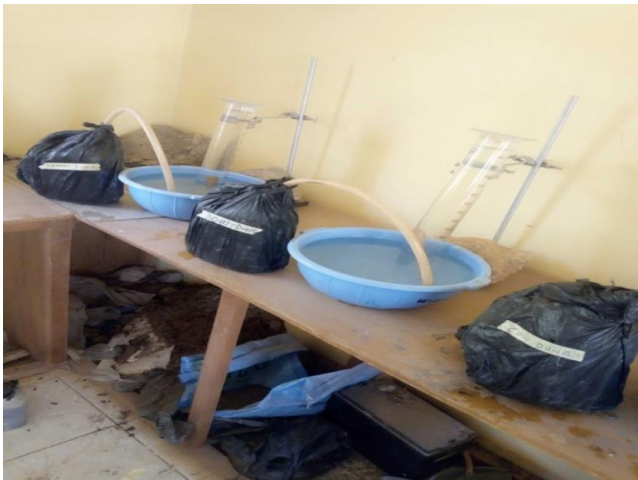
Figure 1: Experimental setups for the comparative production of biogas from selected slurries
